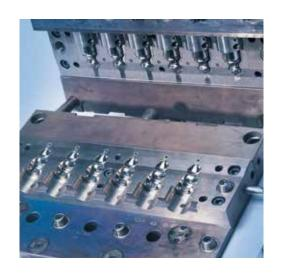
The development of ever-larger plastic parts increases complexity of heat treatments of the moulds. In order to eliminate dimensional changes and quench cracking, prehardened steels are used for large tools.
